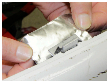
2. Tape the die in place with foil tape.
