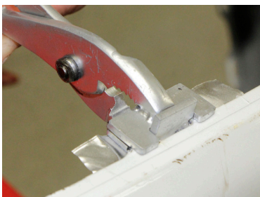
4. Reheat the welded area until soft, then squeeze with die pliers for 30 seconds.
