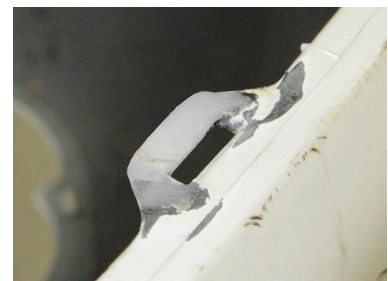
6. Shape the outer edge of the welded bumper to replicate the OEM appearance. Fill and prime with Polyvance products, then paint as needed.
