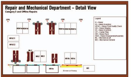
This diagram outlines an area of a facility dedicated to handle the more severely damaged vehicles and mechanical work, and it isn't much different than what we've done for 40 years. The photos below show how the diagram becomes a reality.
