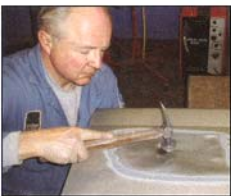
8 Quickly pick up the hammer, and hammer around the hot spot, in the pattern shown below.
