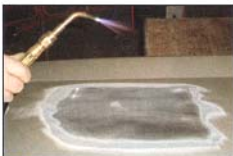
5 Adjust your torch to a neutral JOF (Just Off Feather) flame. The acetylene regulator should be at 5-7 pounds and oxygen at 12-15 pounds. Use a small tip for more control.
