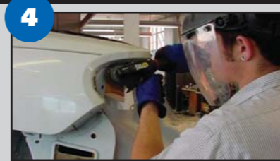
4 Remove all sealant and caulking to expose resistance spot welds that you'll drill out in order to separate the panels.
