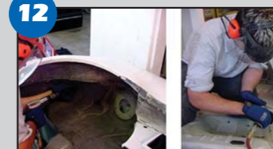
12 Separate the quarter panel with wheelhouse from the rear floor panel and trunk floor to gain access to the spot welds that hold together the inner and outer wheelhouse panels.
