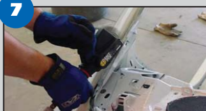
7 Clean off the remaining urethane sealant on the rear window pinchweld.
