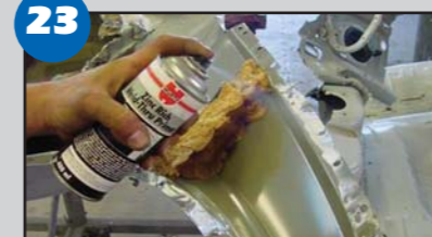
23 Apply weld-through primer to all mating surfaces.
