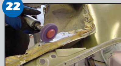
22 Clean up all mating surfaces with special plastic wheel.
