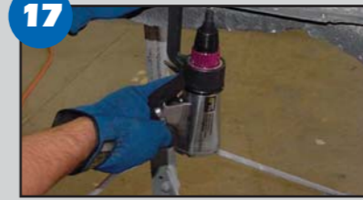
17 Drill out the spot welds that secure the inner and outer wheelhouse panels together.
