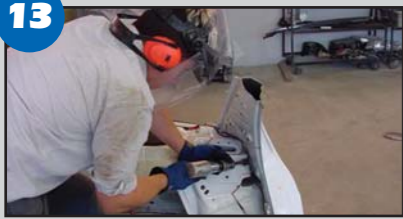
13 Separate the package tray from the quarter panel section for access.
