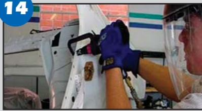
14 Drill out the factory resistance spot welds.
