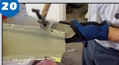
20 Repair all mating flanges with a hammer and dolly.
